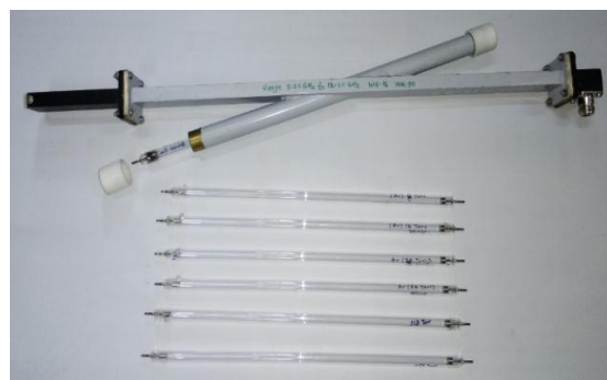
Fig.3 Arrangement for tube mount and photograph of complete noise head mount for X-band with different pressure Argon tubes fabricated (8,16,32,64,128,256 torr)
