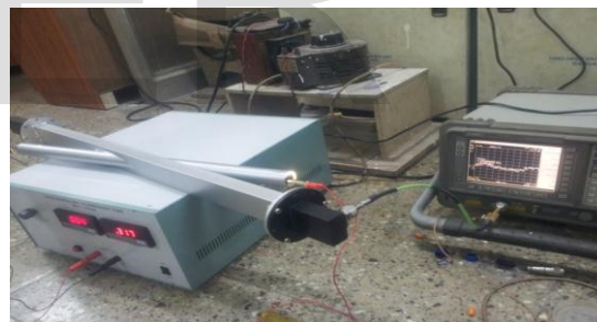
Fig.4 Block diagram and experimental set up for Spectrum Analyzer method of noise power measurement.
